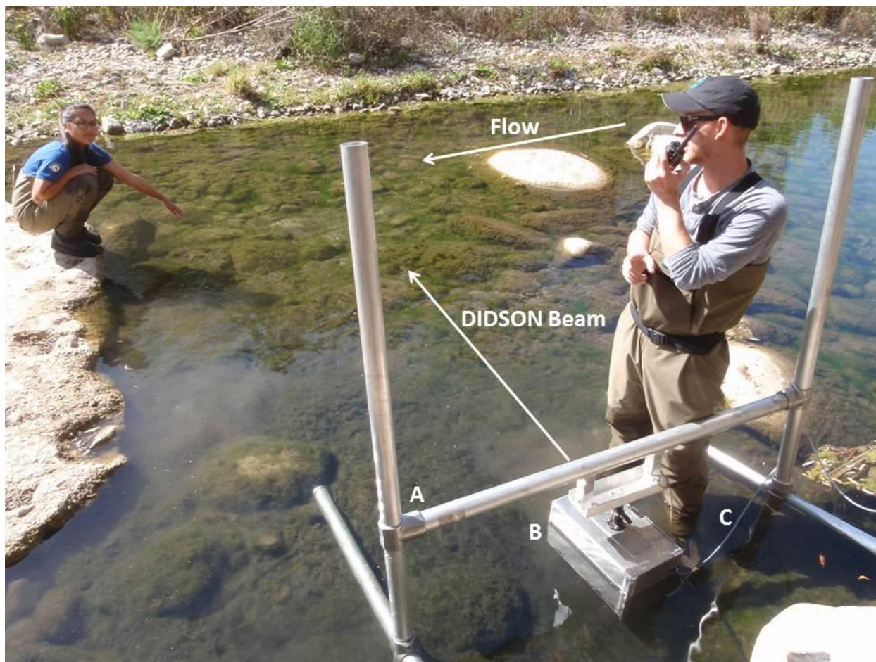
Figure 6. Ventura River DIDSON site in 2013 as viewed from the river left bank. Key features are labeled. (A) H-mount; (B) DIDSON camera housed in both a silt and debris box; (C) security tether.
