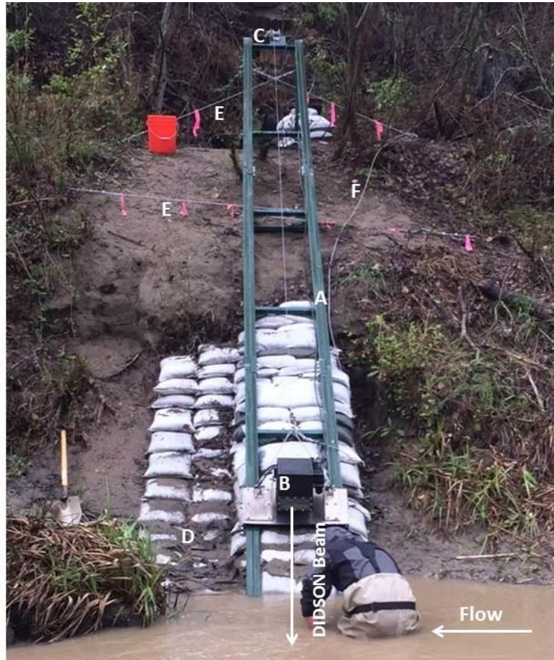
Figure 8. Salsipuedes Creek DIDSON site viewed from across the channel. Key features are labeled. (A) track; (B) DIDSON housed in silt box and mounted to a sled via an X2 rotator; (C) winch used to adjust camera height; (D) gravel bag berm; (E) cross-bracing cables; (F) security tether.
