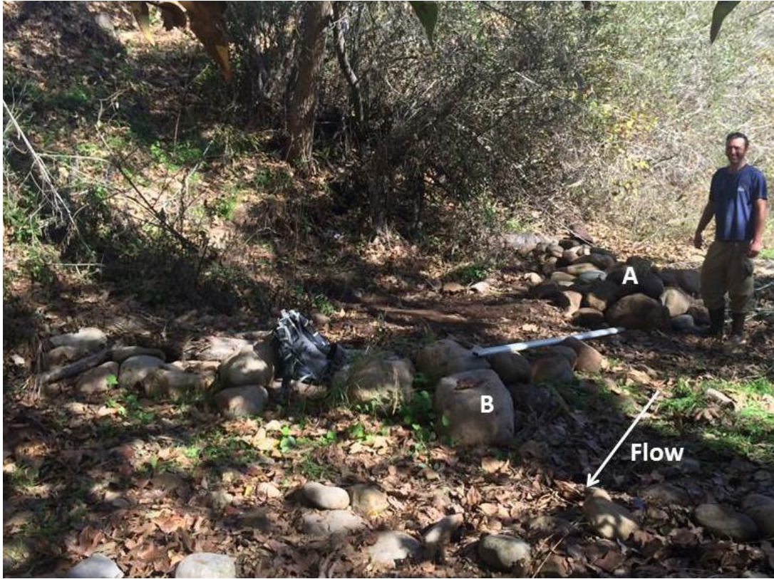
Figure 19. Berms composed of native materials being used to direct fish to an optimal DIDSON imaging range at Carpinteria Creek. Key features are labeled. (A) Upstream berm composed of large cobbles and small boulders; (B) Downstream berm composed of woody debris reinforced with cobbles and boulders.
