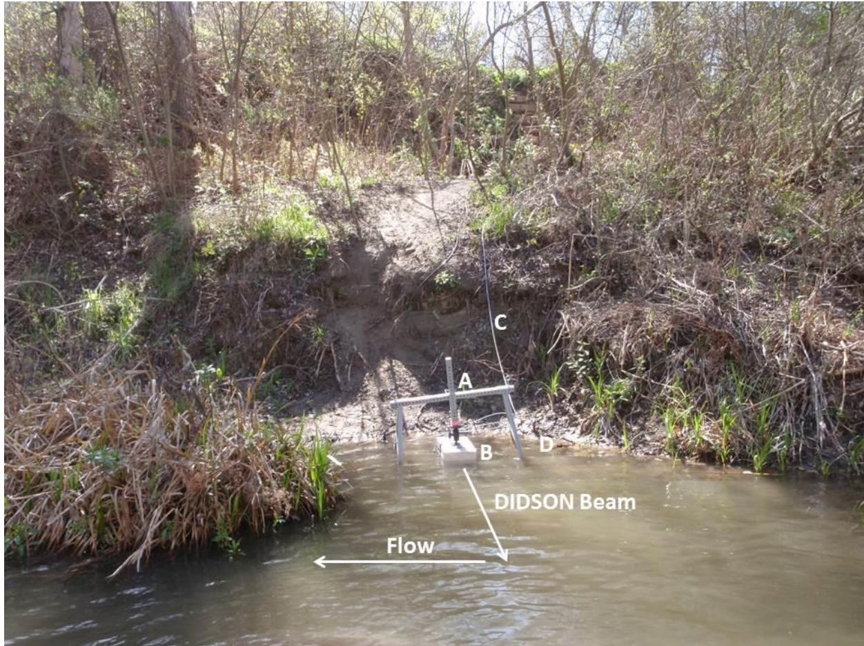
Figure 5. Salsipuedes Creek DIDSON site in 2013 viewed from the opposite bank. Key features are labeled. (A) A-frame mount anchored by gravel bags; (B) DIDSON camera housed in both a silt and debris box; (C) security tether; (D) Earth Anchor.
