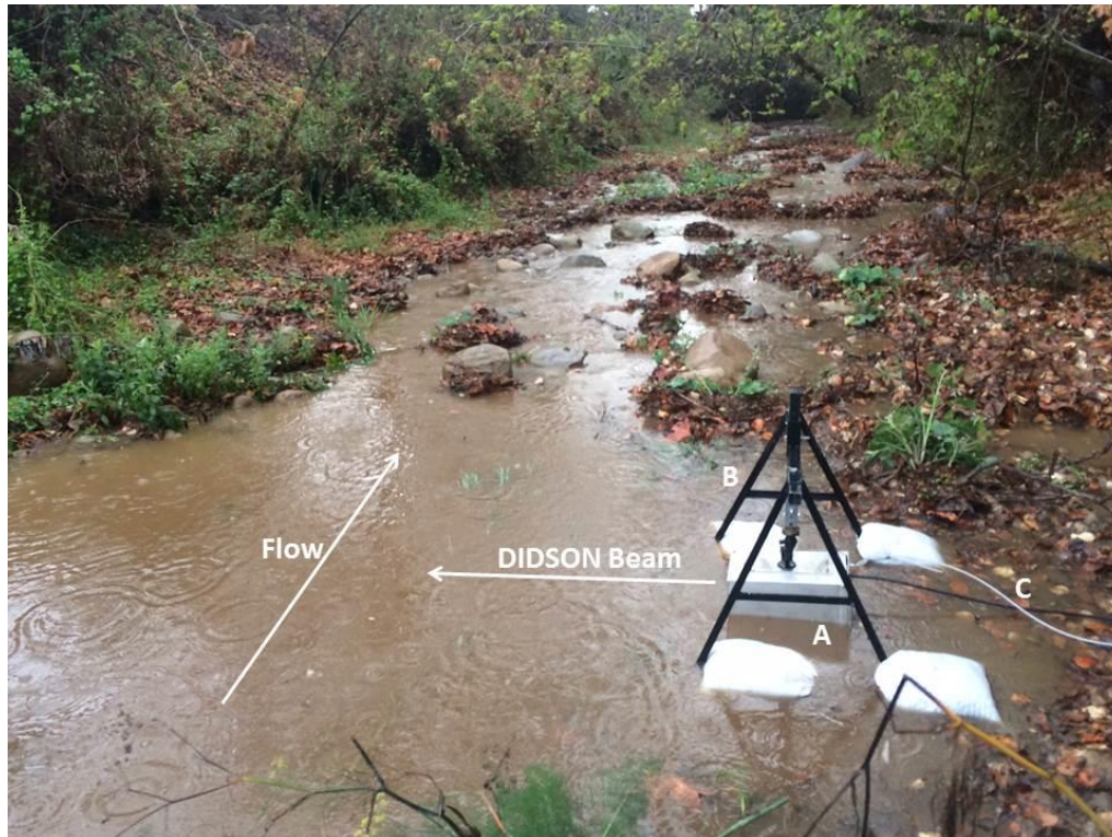
Figure 9. Carpinteria Creek DIDSON site viewed from upstream. Key features are labeled. (A) DIDSON camera housed in a silt box and debris box; (B) A-frame mount anchored by gravel bags; (C) security tether.
