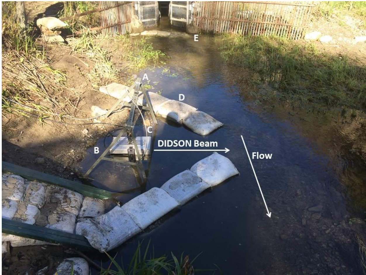
Figure 7. Salsipuedes Creek DIDSON site viewed from downstream. Key features are labeled. (A) A-frame mount anchored by gravel bags; (B) DIDSON camera housed in both a silt and debris box; (C) security tether; (D) gravel bag berm; (E) COMB trap.
